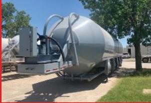
2022-M.Housby specifically 4100 CF portable bulk silo, 477,000 LB capacity, 10-HD screw down legs w/wide footpads, 45 degree sloping hoppers with 8 degree counter Plenums for "total clean out of product", 4" front and rear blow down lines, 3" aeration lines, butterfly valves, 23,500 spring suspension, single 20" manhole with cast pressurized cover, safety ladder, LED lighting, 3 pressure and vacuum relief pop offs, Carboline coatings
