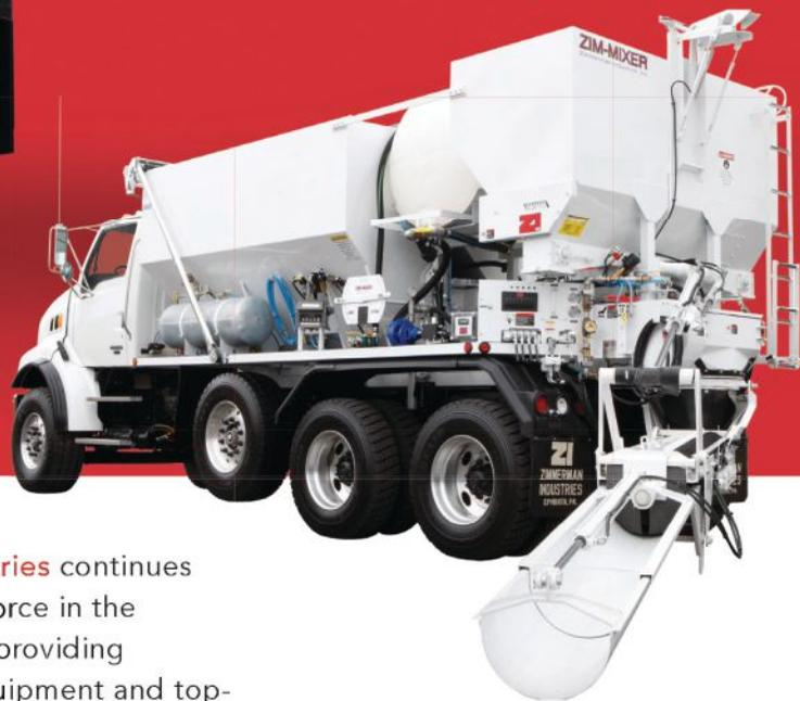
Zim-Mixers® feature patented dual chain material-feed technology that keeps you working three times longer than a belt ever could. Mix an accurate, fresh, custom pour on site, with no waste.
