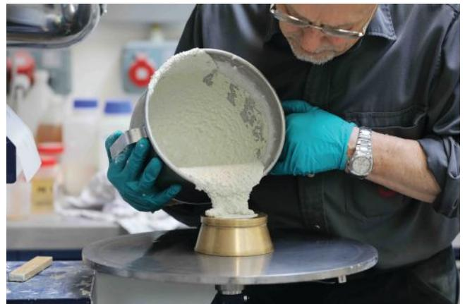
Cementir and Aalborg Portland technical teams cite InBind concrete specimens attaining 24,000 psi compressive strength. Their best performing mixes have been designed with 0.25 water-binder ratio, optimized aggregate packing, and self-consolidating properties.
