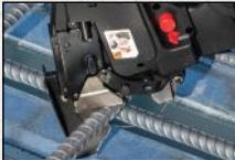
The Wire Pull Back Mechanism dispenses the precise amount of wire needed to form a tie.
