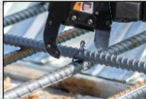
The TwinTier's Wire Bending Mechanism produces a shorter tie height. Less concrete is needed to fully cover a wire tie.
